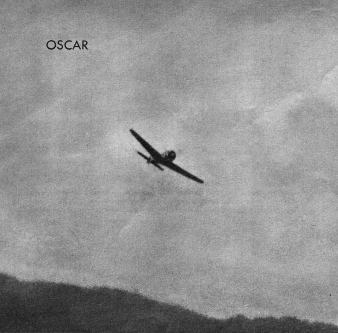
Short nose on Oscar ( above and below ) is its most striking recognition feature. Fuselage by contrast seems long and slender as wing is set far forward. Oscar is an Army fighter, used mainly in the Burma-India theater. The Mark II has a new engine, span 2 ft. less and blunter wingtips.
